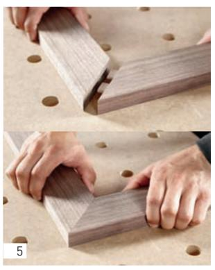
Insert the dominos, using a sufficient amount of glue, join the frame rails and brace them with clamps.
