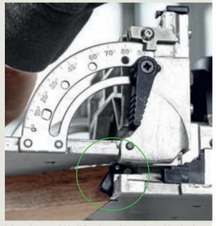
It is easiest to quickly define the positions of repetitive domino holes by using the integral stop catches for both parts of the workpiece. The distance between the stop catch and the router centre is 37 mm. Place the DF 500 at the edge of the workpiece using a stop catch.
