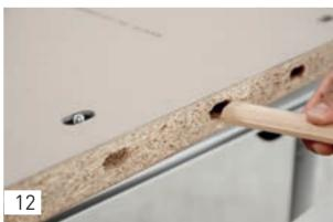
If you have decided to use additional dominos in order to ensure a flush connection and extra transverse load transmission, insert these into the other routed holes.
