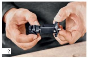
To fit the cross stop on the machine in question, turn the clamp jaw on the stop pin so that it is set to the DF 500 or DF 700 position (each machine is marked accordingly on the front of the pin).
