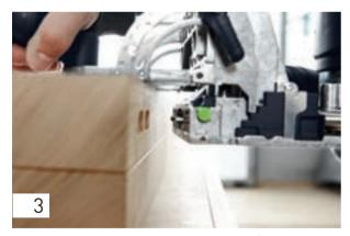
Route the domino holes in the table or bedpost (narrow hole width) with a routing depth of 25 mm. Set one hole for the expansion bolt of the corner connector, the others for the load transfer via traditional dominos.
