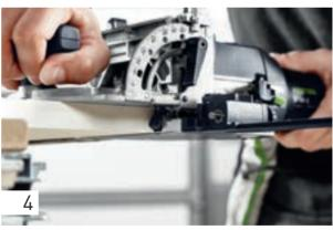
For this reason, a routed hole with a depth of 25 mm is created (on the front side) for this butted joint. The other routed hole (on the surface) is 15 mm deep, so that the total domino length of 40 mm is processed.
