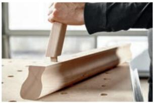
Set the routed holes in the handrail as described above. Then join the spindle and handrail together.
