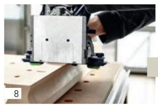
Route the holes in the handrail, positioning the joining machine on the second marking.
