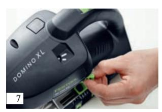
Switch the machine to the large hole width for the transverse holes; this gives the transverse anchors enough space when fitted with the enlarging clips.
