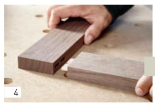
Use this method to carry out routing for all four frame rails, whereby every second frame rail is routed into the workpiece lengthwise instead of into the front.
