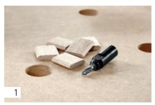
To process the smallest domino  $(4 \times 20 \text{ mm})$ , insert the 4 mm router into the DOMINO DF 500. This router is unique in that it is shortened by 10 mm. Therefore, at the maximum routing depth of 20 mm, the routed hole is only 10 mm deep.
