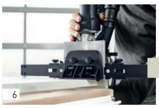
Use the same process to create the routed holes for the side wall of the cabinet. Set the first hole with the stop pin of the DOMINO joining machine...
