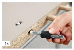
Then push the double-headed bolt into the workpiece...
