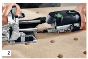
Separate the motor unit and guide frame.
