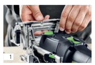
Set the routing height to match the thickness of your workpiece. For the routing depth, select half the domino length. Route the holes by either using the right hole width for both for extreme precision fit or routing the second hole with clearance, if desired.
