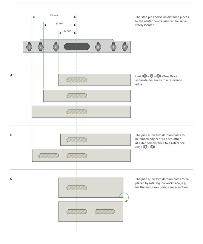
Additionally, it is possible to insert the pin in the previously routed domino hole and to use the edge of the domino hole as a stop. This means you can define domino holes over larger, uniform distances independent of the edge of the workpiece and without marking. (In the example using pin 2 in the drawing.)
