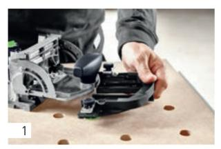
Mount the trim stop onto the DOMINO joining machine according to the operating instructions.
