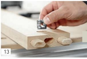
The transverse anchor is then inserted into the transverse hole in the side wall, with the screw hole facing upwards.
