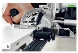
For the other routed holes, set the desired hole distance on the cross stop and position the pin in the first routed hole. Route the other holes as slots.
