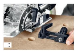
Mount the cross stop onto the joining machine according to the operating instructions. In this example, we are processing 6 x 40 mm dominos.
