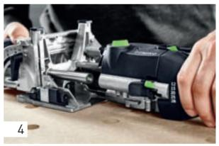
Before inserting a new cutter, ensure that the machine, the guide frame and the guides are clean and free from chippings. Remove any soiling. Only use sharp, undamaged and clean cutters. Now push the guide frame onto the motor unit until it audibly locks in place.
