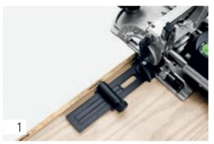
With larger workpiece widths and larger hole distances, the cross stop can be used to work easily with the stop pin system instead of marking out holes.
