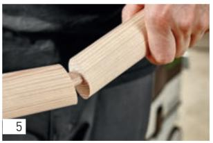
Insert the  $8 \times 40$  mm domino into the routed hole, applying glue to the joint. Then join the two workpiece parts together – the joint is secured from twisting with just one domino!
