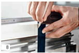
Then create the routed holes for the shelves (this process is similar for carcass sides etc).
