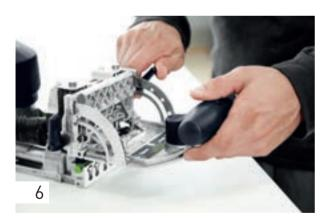
The flip stop point, i.e. the routing height adjustment, must always be set to 40 mm. This ensures that the transverse hole always sits at the right distance to the edge of the workpiece and that the anchor bolt then catches the transverse anchor.
