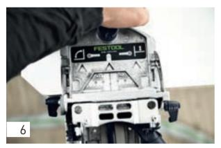
Route the 50 mm deep holes with the narrow hole width into both workpieces at the markings. The joining machine is placed on the top side of the worktop in this case.
