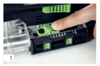
Set the routing depth of the joining machine to 25 mm – set the markers to 25 mm and 50 mm.
