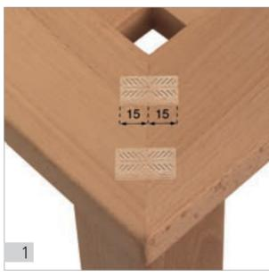
In this example, we are processing 5 x 30 mm dominos. Set the routing depth to 15 mm for this.
