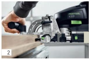
In the lengthwise rail, set the routed holes with a 70 mm routing depth as well, but route the first hole with precision and the second as a slot with clearance. Proceed likewise for the additional lengthwise and crosswise rails.
