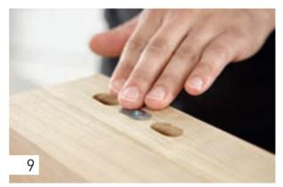
It is important to ensure that the expansion bolt is flush with the workpiece surface.
