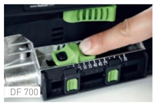
**DF 700** Press one or both locking switch to set the routing depth. Move the routing depth setting slider to the required routing depth. On the DF 700, the possible routing depth is between 15 mm and 70 mm. Now release the locking switchbriefly check that the slider has locked in to position.
