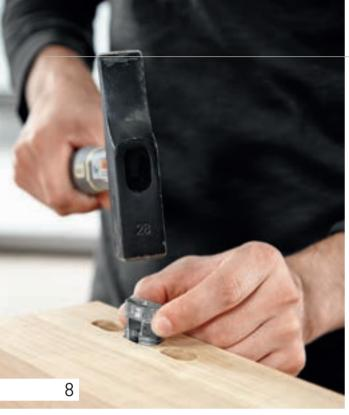
Insert the expansion bolt into the centre routed hole in the post.
