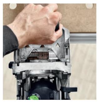
**DF 500** It is possible to define the positions of the DOMINO routed holes by simply drawing and locating the machine on the scribe mark looking through the viewing window.
