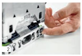
Use the stop pin system to select the hole distance based on the individual workpiece. In this example, we are working with the two centre pins, to create a hole distance of 37 mm.
