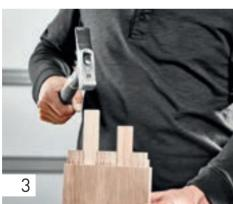
Then cut the dominos to fit the ready-made holes. In this example, the nominal domino length is 115 mm, which is calculated by doubling the routing depth of 70 mm = 140 mm and subtracting the pinned joint of 25 mm = 115 mm. Cut the domino a few millimetres shorter (so that later the glue has enough space), down to 112 mm. Chamfer the cut domino at the edges using a sanding block.
