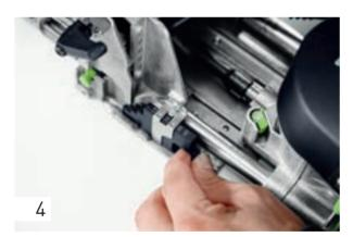
Set the routing height: the distance from the flip stop to the centre of the router should be half the worktop thickness. With a worktop thickness of 38 mm, for example, set the routing height to 20 mm.
