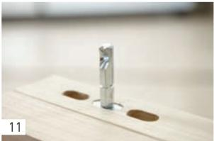
Then unscrew the bolt just enough so that the countersink is facing the right direction. The expansion bolt is now sitting securely in the workpiece and cannot fall out of the routed hole, even if the joint is disassembled for transport purposes.
