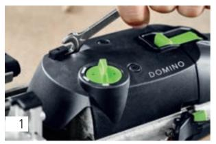
Always disconnect from the mains to change the cutter. Then raise the unlocking lever using an open ended spanner (included) until it noticeably locks in place.
