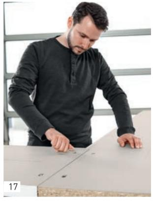
$\ldots$  and clamp the connectors by tightening the stud on the second workpiece side.
