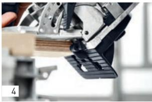
Flip the additional stop pin from the additional stop and place the joining machine on the workpiece – the routed holes will be further offset from the edge of the workpiece, which is beneficial with such narrow workpieces.
