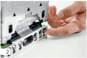
It is a good idea to work with the stop pins in this case. Select the pins depending on the desired hole distance. Ensure that the routing for the corner connector has a minimum distance of 37 mm from the edge of the workpiece. If you work with the stop pins, use the centre pin at least.
