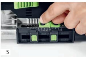
Then set the routing depth to 50~mm and set the markers to 50~mm and 30~mm.
