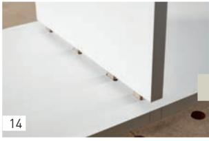
Proceed likewise for the second side part. Then insert the domino in the routed holes and join your workpiece together, applying glue to the joint.
