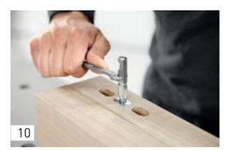
Then screw the anchor bolt all the way into the expansion bolt. This expands the expansion bolt, pulling it another approx. 1 mm into the workpiece thanks to the self-drawing property of the bolt and locking it securely into place. A 10 mm open ended spanner is used for this.
