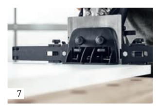
$\dots$  and create the others using the cross stop pins. Using the additional stop, along with the cross stop – is beneficial here, because the joining machine has a sturdy support surface on the panel.
