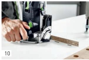
In our example, the centre shelf and side part are flush at the front and are clamped accordingly. Adjust the angle of the joining machine to 0° and the routing depth to 15 mm. Then route the first domino hole with the narrow hole width with the stop pin in the horizontal side part.
