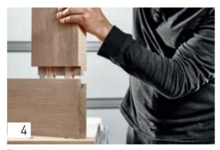
Then drive the dominos all the way into the routed holes in the end grain, adding glue to the joint.
