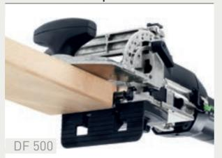
The additional stop provided with the DF 500 increases the contact area and reduces the lateral distance of the stop catches to the DOMINO centre from 37 mm to 20 mm. This allows precise positioning of narrow workpieces.
