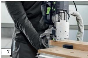
Then route the transverse hole into the frame, where the connector will be inserted. Flip the handle down at the front of the edge of the workpiece and align the machine at the scribe mark or using the stop pins (depending on how the horizontal routed hole was set).
