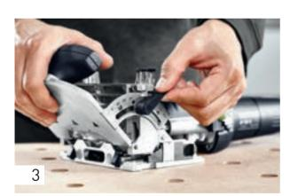
Set the routing depth to 20 mm, the routing height to the minimum and the routing angle to 45°.
