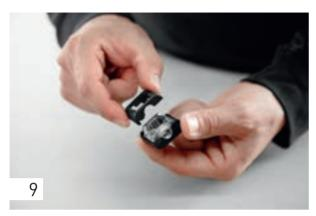
The enlarging clips around the transverse anchors prevent the anchors from drawing into soft materials (e.g. kitchen worktops) when tightened. Clip the enlarging clips around the transverse anchors for this purpose.
