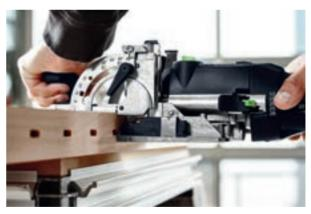
Set the routing height to the centre of the workpiece. Mark out the axis distance of the spindles on the top side of the workpiece. In this case (when simply using markings) bring the scale in the viewing window of the DOMINO over the scribe mark and set the routed holes. A second scribe mark, as in the example of the handrail above, is not necessary here.
