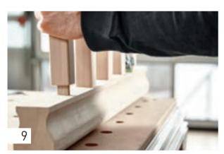
Applying a sufficient amount of glue, insert the dominos into the routed holes and join the handrail to the spindles.
