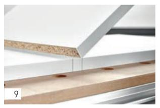
Place the top side part to one side. Position the centre shelf at the marked point and fold it over towards the right or left, so that the top or bottom edge of the centre shelf is aligned with the corresponding marking. Clamp both workpieces (centre shelf and side part).
