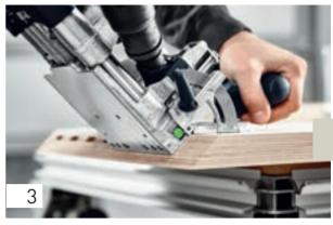
After routing the first hole (the pin is positioned at the edge of the workpiece in this case), the pin goes into the routed hole, thus setting the next stop. Route the first hole with precision, and all other holes as slots with clearance.
