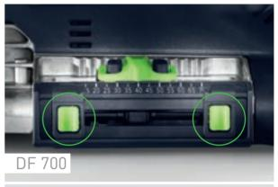
TIP You can mark two routing depths using the two green markers and easily move between the two using the slider. For example, this can be helpful when using a domino depth for spacing as well as for repeated, identical routing depths.
