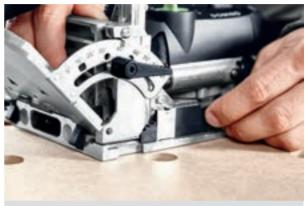
TIP Route thin workpiece with a mitre. Set the required angle. Loosen routing height adjustment clamping lever, push the slider towards the motor unit until it stops and then push the angle stop all the way down. Close the clamping lever.
