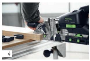
Change the routing depth to 50 mm and route the holes (narrow hole width) in the frame according to the scribe mark or using the stop pin system. The routing height is determined by the material thickness, using the usual method you already know from working with your DOMINO DF 700. In this example, the frame has a material thickness of 30 mm. Set the routing height to 15 mm so that the routed hole is centred in the material.
