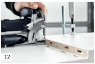
Switch the routing depth to 25 mm and route the domino holes in the centre shelf, again using the stop pin for the first routed hole (narrow hole width).
