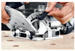
**DF 500 and DF 700:** Loosen the angle stop clamping lever to adjust the routing angle. Then set the required angle, either continuously on the scale between  $0^{\circ}$  and  $90^{\circ}$  or in stages at  $0^{\circ}$ , 22.5°, 45°, 67.5°, 90°. Close the clamping lever.
