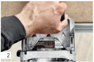
The routed holes can be set by marking them out as usual or using the stop system with the scale in the viewing window – in this example, 15 mm from the outside edge. For this option, place the scale with the 15 mm marking at the edge of the workpiece.
