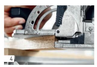
For the second routed hole, either mark out the position or run the machine flush along the outside tip of the mitre. This routed hole can either be precisely routed like the first hole – which increases the stability of the joint but requires more precision – or it can be routed with clearance – but then you must use a sufficient amount of glue for the joint.
