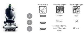
Only suitable for joining timber or timber-like materials in furniture construction (no lightweight building materials!) The DOMINO connector is only a connecting element, not a load-bearing element. Observe minimum routing depths and edge distances! For indoor use only!
