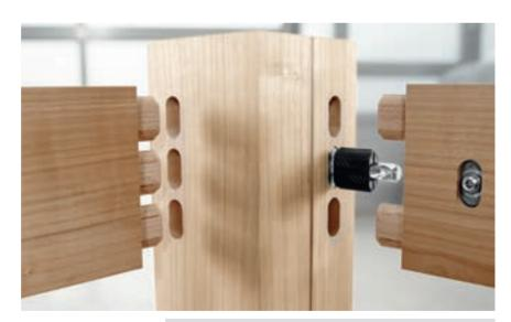
**TIP** It is usually a good idea to fit flexible connectors to one of the sides and securely glue dominos into the other side.
