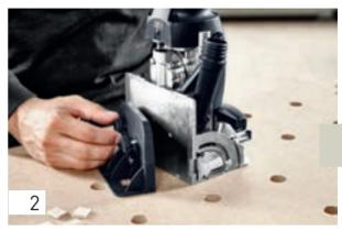
Set the additional stop on the DOMINO DF 500. This uses the additional stop pins to reduce the lateral distance to the centre of the DOMINO router from 37 mm to 20 mm.
