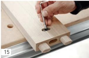
Then insert the threaded screw. Tighten it only so that the screw stays in place, but the opening remains open for the anchor bolt.
