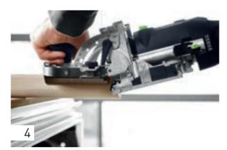
Set the routing angle on the joining machine according to your sawing angle on the workpiece. In our example, the handrail was sawed at 15°, which means the routing angle is set to 75°; this is equal to 90° minus 15°. Secure the workpiece, on the MFT multifunction table. Then route the hole in both parts of the workpiece.
