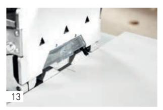
Set the other holes using the scale in the viewing window, which you align with the scribe marks. Set all holes here in the panel edge with the narrow hole width – the domino will be glued here first and will then fit in precisely.
