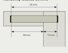
TIP The domino should generally be centred within the joint; that is, the routing depth should correspond to half of the domino length. However, depending on the workpiece or joint type, it may be necessary to locate the domino randomly. In this case, both of the holes routed in the workpieces must together correspond to the length of the domino being used.
