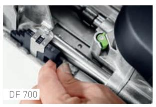
**DF 700** The routing height is adjusted on the DF 700 equivalent to the DF 500. The only difference to note: here, the preselect setting does not determine the board thickness, but instead the true distance from the top of the workpiece to the centre of the routed hole.
