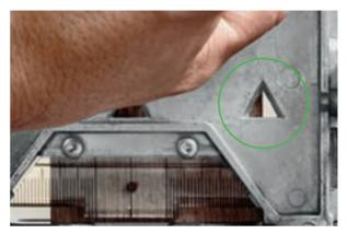
The edge of the workpiece is visible in the machine's upper triangular viewing window. If you do not need the stop catches, they are automatically pushed aside during the routing process.
