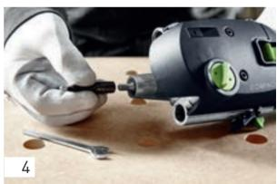
To process a  $6 \times 40$  mm domino as in this example, use the 6 mm router (6 mm dominos can only be processed with the DF 500). For details on changing the router, see chapter 1.4.4, page 18.
