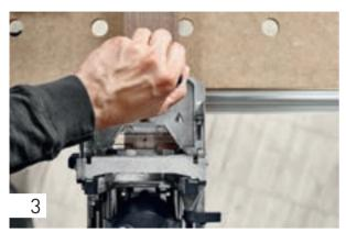
The second routed hole is set here using the stop catch. This method makes it possible to position two dominos next to each other working from just one reference edge.
