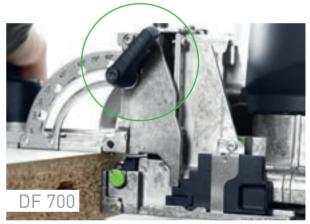
NOTE The alignment of the clamping levers can be adjusted by lifting them. In the tightened state, they should not overhang past the contact surface.
