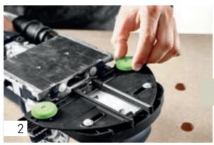
Set the width of the trim stop to the thickness of your spindle by adjusting the guide in the parallel side fence to the correct dimension using the scale and the green rotary wheels. In this example, we are working with 30 x 30 mm rectangular spindles.
