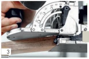
We are using two dominos per corner connector for maximum stability. Place the routing machine on the mitre cross section and carefully work with the stop catch at the side against the tip of the mitre. Route the first hole with precision.
