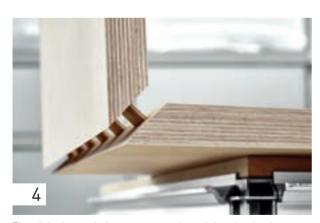
Then join the workpiece parts together, gluing the dominos carefully in the process.
