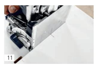
For the other domino holes, switch the hole width to the slot and mark out the domino positions with a simple scribe mark on the horizontal centre shelf. Then place the joining machine on the scribe mark. Use the markings placed on the bottom of the joining machine by positioning the centre marking on the machine at the scribe mark on the shelf.
