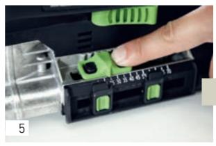
Then set the routing depth to 25 mm for routing the transverse hole. (This dimension depends on the workpiece; see dimensional drawing. What is important to note is that the transverse hole should overlap the longitudinal hole by 3 mm in depth.)
