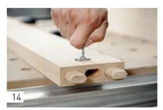
Press the transverse anchor all the way into the routed hole using the spanner.
