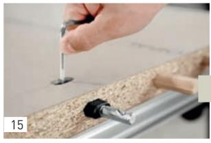
... and tighten the stud in the first transverse anchor.
