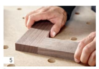
Then glue the frame rail and brace with pads and clamps, if necessary.
