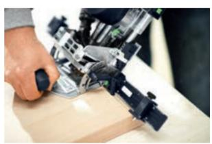
TIP For larger hole distances, you can work with the cross stop (available as an accessory or included in the DF 500 set) both with the DF 500 and the DF 700.
